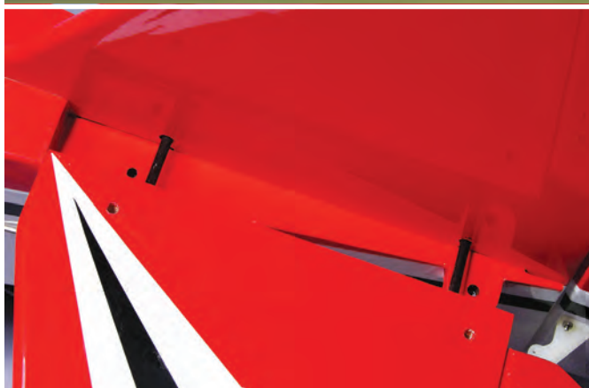
The stabilizer halves slip into place using a system similar to removable stabilizers on larger aerobatic models. Two rods pass through the vertical fin to align the halves. Everything is held in place with four bolts.
