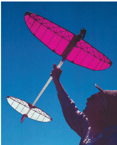
Sunlight accents the wing and stabilizer structure of Bob Mattes' new E-36 model. Even the molded fiberglass fuselage seems to glow.
